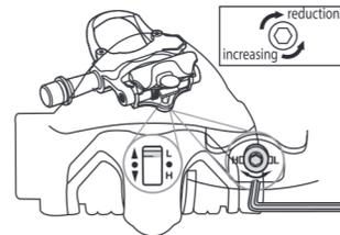
For the increasing of spring preload turn the adjusting screw clockwise.
